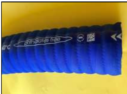
Blue cover, white lining Corrugated Non-Toxic - Non-Tainting EPDM rubber with polyester plies Temp Range : -30°C to +140°C 4 : 1 Burst Pressure Safety Factor
