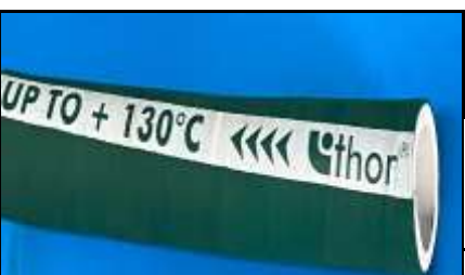
Crush resistant Nylon Helix Suction hose for Milk, Wine & Beverage, FDA & USDA Approvals. Temp Range : -31°C to +130°C 4 : 1 Burst Pressure Safety Factor
