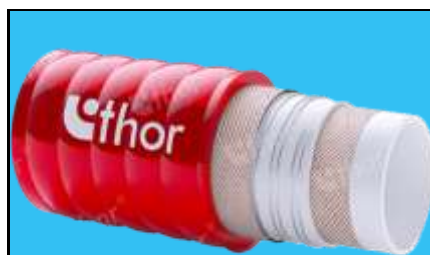
Red cover, white lining Corrugated Non-Toxic - Non-Tainting Butyl rubber with polyester plies. PE film coating on outside. Temp Range : -30°C to +130°C 4 : 1 Burst Pressure Safety Factor
