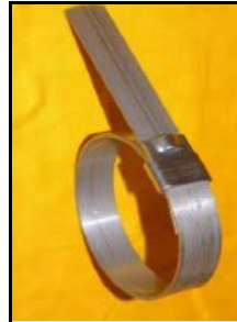
Extremely strong Pre-Formed 2 ply band clamps. Extra Thick Stainless Steel 201 series, with HD Ultra Lok Buckle. Needs Ultra Lok Tool for fastening.
